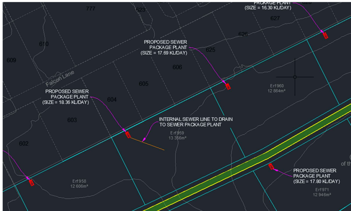
Figure 4: Internal Sewer connections
