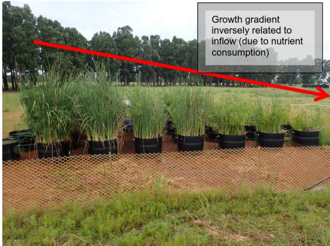
Figure 1: Typical arrangement for a vertical reed bed post purification.
