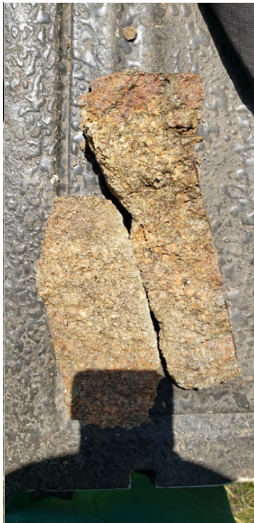
Intact, highly weathered, soft rock granite
