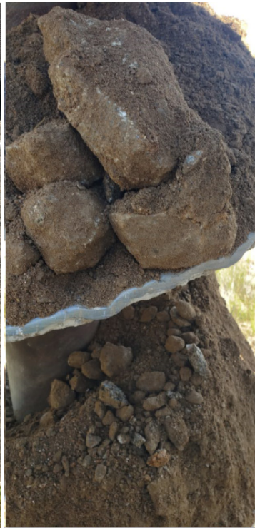
Pulverised soft and medium hard rock granite on the auger flight
