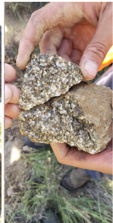
Significantly less weathered, medium hard rock granite
