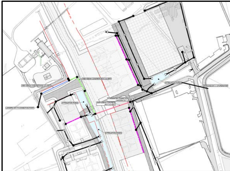
FIGURE 22: PROPOSED STORMWATER PLAN AND ATTENUATION AREAS
